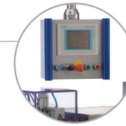
**Control panels** can be programmed to adjust the blister strip length, production speed and manual/production modes
